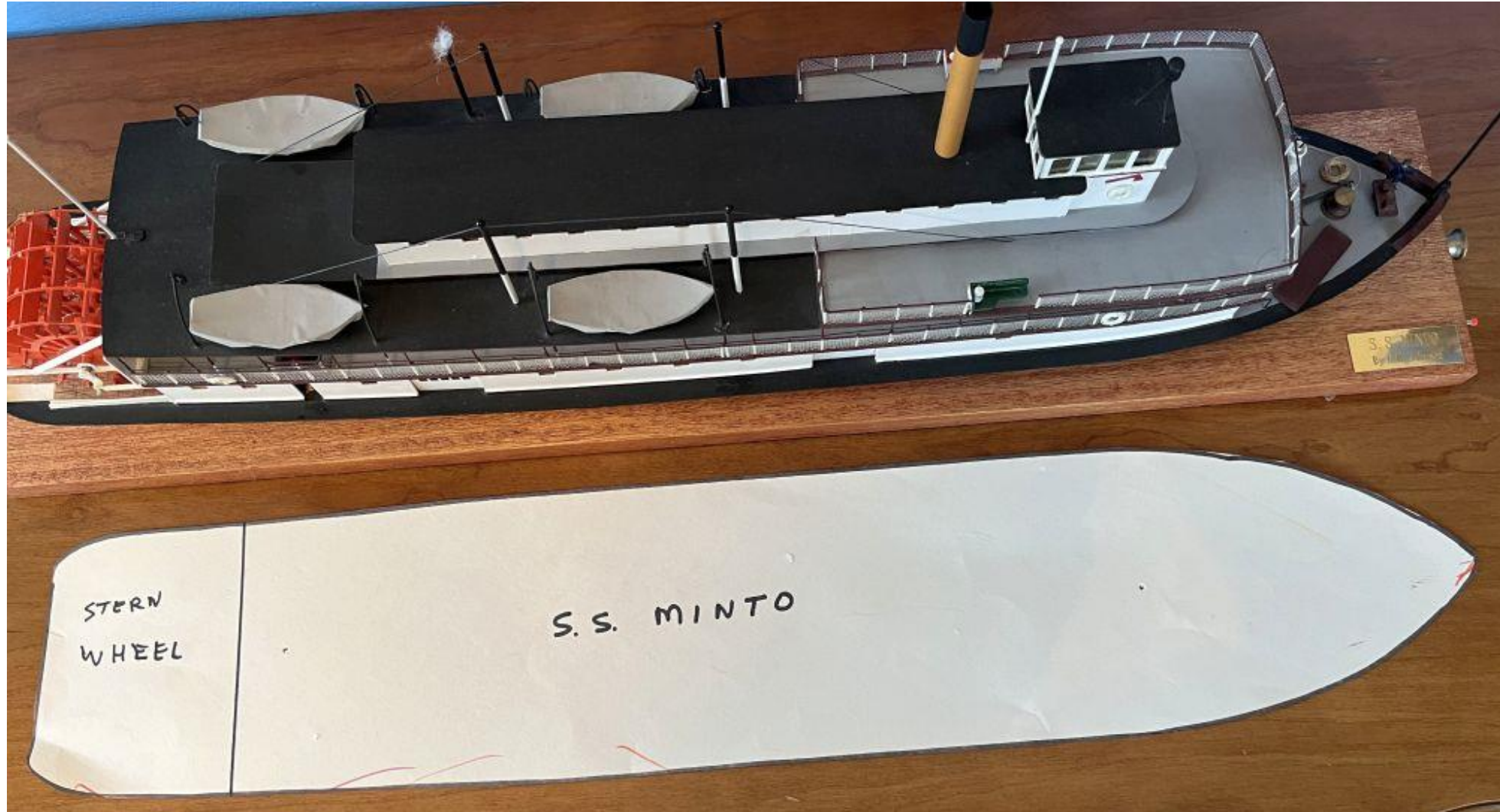
The hull pattern shown alongside the finished boat.
